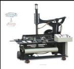
Finished Case Size(minimum): 100X80X15(mm) Finished Case Size(Maximum): 360X500X100(mm) Capacity:20-40pcs/min Power:1HP/380V
