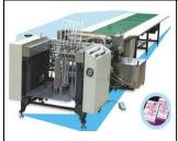
Sheet width:80-600(mm) Sheet thickness:80-200(g) Capacity:7-40pcs/min Power:3HP/380V
