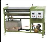
Maximum sheet width:700(mm) Sheet thickness:80-300g Coating thickness:0.2-3.5(mm) Capacity:23m/min
