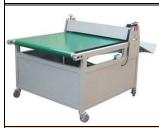
Finished Size: 900(mm) Maximum Capacity: 50 Pcs/Min Power: 1HP/380V
