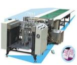
Sheet width:80-600(mm) Sheet thickness:80-200(g) Capacity:7-40pcs/min Power:3HP/380V
