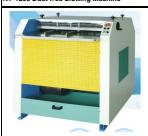
Applicated width: 50-1100mm Applicated longth:50mm-unlimited Gap bewteen two slots: 0-900mm Applicated thickness: 0.8mm-4.0mm slotting Number:Max 8 (customize) Speed: 10-35m/min Power:3.7KW/380V
