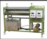
Maximum sheet width:700(mm) Sheet thickness:80-300g Coating thickness:0.2-3.5(mm) Capacity:23m/min Power:5KW
