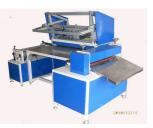
Thickness: 80---350gsm Min size: 60x60mm Max size: 450x900mm Power: 1.2kw Voltage: 220v/50hz Speed: 120-200pcs/hour Air compressor: 0.6Mpa Weight: 320kg
