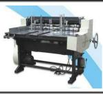
Maximum Width: 1200(mm) Thickness:1-4(mm) Capacity: 75m/min Power:1.5KW
