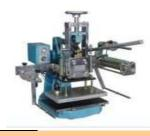
. Stamping Size: 400\*600 mm (16\*24 inch) Working table area: 800\*520mm Max printing pressure: 15, 000 Kg Up and down distance: 70mm
