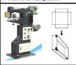
Minimum finished Case size: 40X40X10(mm) Capacity: 1pcs/sec Power:0.5HP/200V
